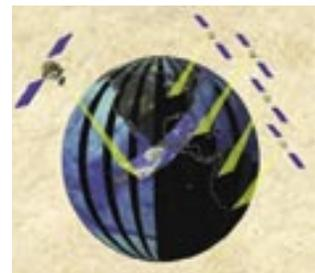
The Global Precipitation Mission (GPM) is designed with a core satellite flying with a constellation of satellites to provide accurate global estimates of horizontal and vertical structure of rainfall and microphysics elements.
