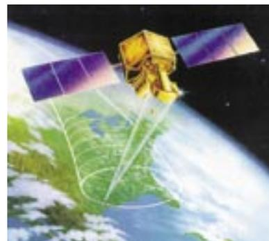
Global Wind Explorer – A mission concept to directly observe the dynamics of the atmospheres using a Doppler lidar to profile wind in the troposphere and stratosphere.
